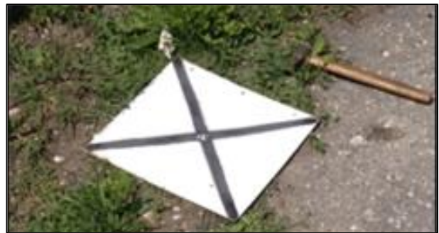
Figure 3.10. Ground control point marks
