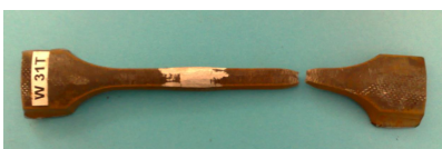
Fig. 5.104. Epruvete rupte W3T [117].
