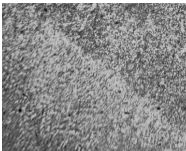
Fig. 5.99. Proba E3T, ZIT, atac Nital 2%, 100X [117].
