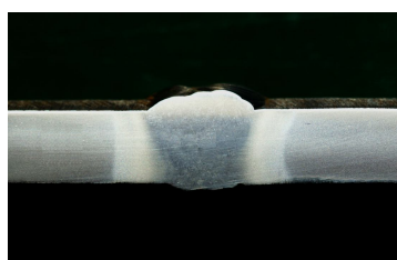
Fig. 5.106. Proba W3T, Atac Nital 10% [117].
