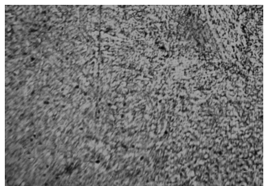
Fig. 5.112. Proba W3T, ZIT, atac Nital 2%, 100X [117].
