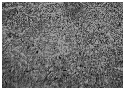
Fig. 5.110. Proba W3T, SUD, atac Nital 2%, 100X [117].
