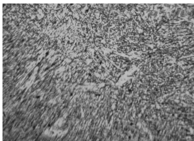
Fig. 5.109. Proba W3, SUD, atac Nital 2%, 100X [117].
