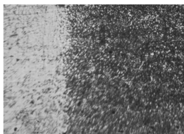
Fig. 5.125. Proba F3T, ZIT, atac Nital 2%, 100X [117].
