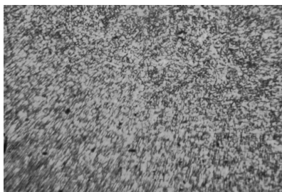
Fig. 5.111. Proba W3, ZIT, atac Nital 2%, 100X [117].
