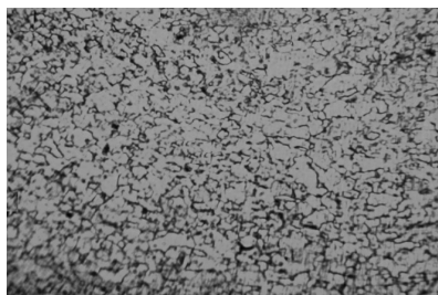
Fig. 5.108. Proba W3T, MB, atac Nital 2%, 100X [117].
