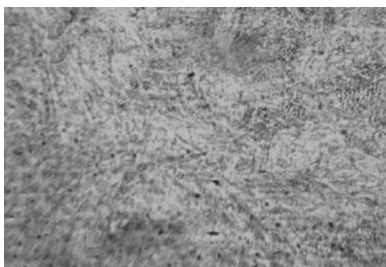
Fig. 5.122. Proba F3, SUD, atac Nital 2%, 100X [117].
