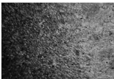
Fig. 5.124. Proba F3, ZIT, atac Nital 2%, 100X [117].
