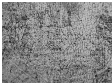
Fig. 5.123. Proba F3T, SUD, atac Nital 2%, 100X [117].
