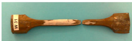
Fig. 5.103. Epruvete rupte W3 [117].
