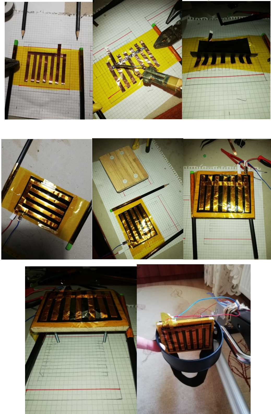
Figure 7.22 Building and mounting the sensor on the hard MDF platform of the pedal [own contribution]
