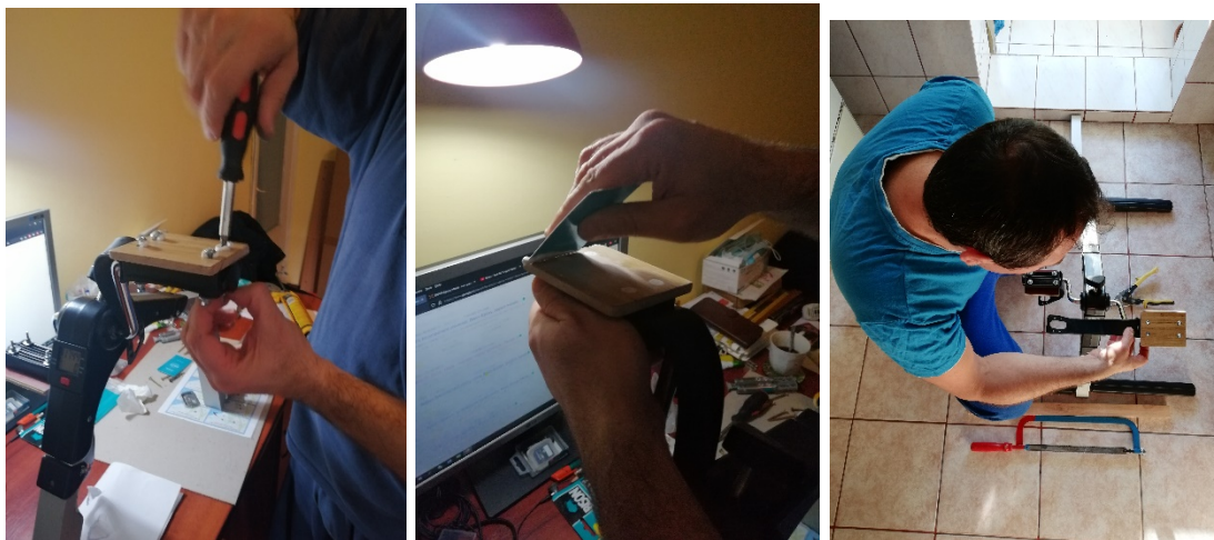
Figure 7.20 Support devices - hard pedal platform for pressure sensor - MDF [own contribution]
