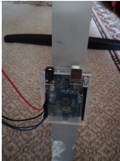
Figure 7.24 Assembly of the Arduino UNO R3 CH340 board [own contribution]
