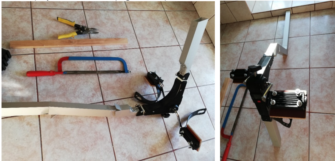
Figure 7.17 Arms made of aluminum profile attached to the pedal [own contribution]
