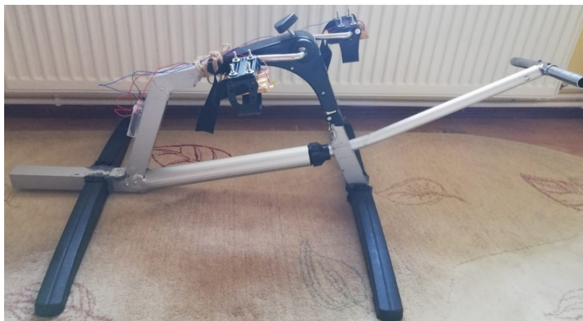
Figure 7.25 Entire horizontal pedal assembly [own contribution]
