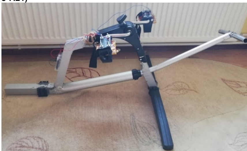
Figure 7.21 Construction and installation of the central axis for balancing and supporting the telescopic handlebar [own contribution]
