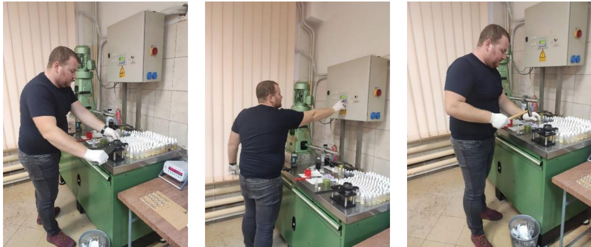
a) Ball cup preparation b) Adjustment of the working regime (time and velocity) c) Extraction of lubricant and balls from the cup, after testing
