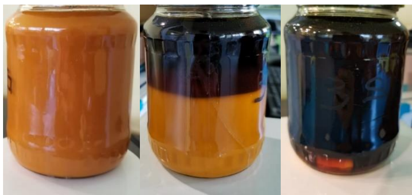
Fig.3.3. Mixture for sample formation with metal chlorides C in day 1, day 31, day 51 (from the left to the right)
