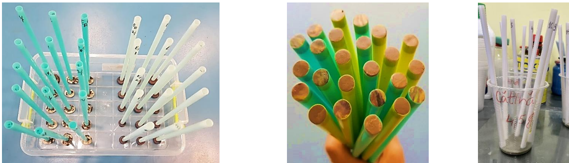
Fig. 1. Polypropylene tube molds with plasticine plugs
