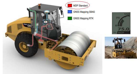
Fig. 2.11. Implementation of MDP technology [38]
