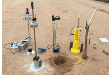
Fig. 2.2 Common devices for in situ measurements of soil properties with: light weight deflectometer, dynamic cone penetrometer, Clegg hammer, test plate
