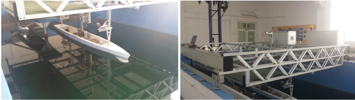
Figure 4.31 Ship model and the towing carriage arrangement
