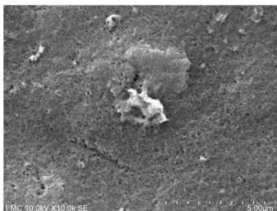
Figure VIII.2 Scanning electron micrograph of the active surface of CNT-GNP-Lac/SPCE
